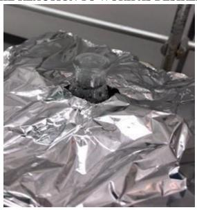
**3.** Center the flask so the stir bar stirs evenly at setting 5 or 6, then heat at 300°C (NO preheating) for 5 minutes.
